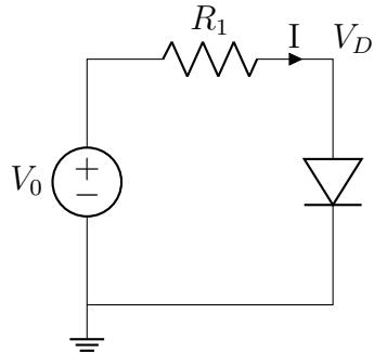
KVL tells us that the sum of voltage drops around a closed loop must equal 0. As such, if we apply KVL.
