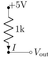
From this, it is clear to see that no current flows, and  $V_{\text{out}}$  sees the entire  $5V$  that is being supplied.
