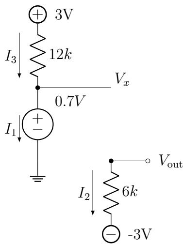
If  $D_1$  is forward biased, we replace it with a voltage source of  $V_F = 0.7V$ ,  $D_2$  we replace with an open circuit.
