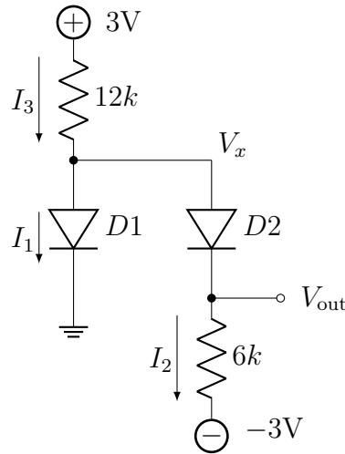
In this example there are two diodes. For each diode we need to assume a forward bias and a reverse bias, checking conditions for each. Thus, we have the four cases:
