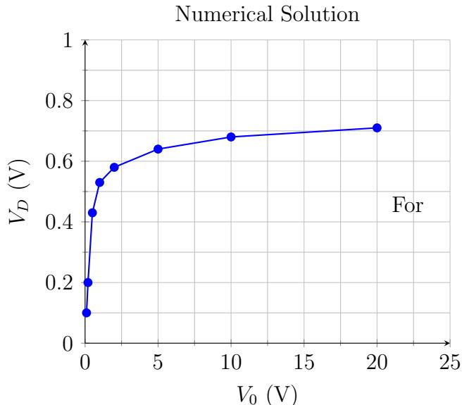
$V_0 < 0.5\text{V}$ , we can see that the current is limited to low values by the diode and there is little voltage drop across the resistor.
