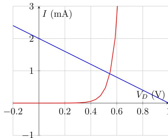
The solution can be read from where the two traces intersect.
