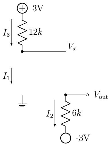
Assuming a reverse bias for each diode, we replace the diodes with open circuits.
