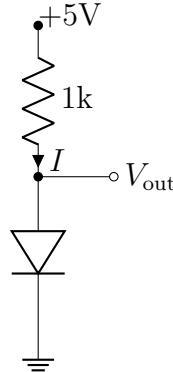
First we will assume that the diode is forward biased. Meaning, we assume the anode is at a higher voltage than the cathode.
