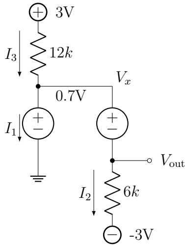
Assuming a forward bias for each diode, we replace the diodes with a voltage source,  $V_F$ . Solving this circuit we find that  $V_x$  is at a voltage of 0.7V. Similarly,  $V_{\text{out}}$  is at a voltage of 0V. This is because the diodes, which were replaced by voltage sources, hold those nodes at the voltages dictated by the forward voltage of the diode.
