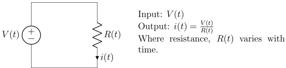
$$\begin{array}{c} v(t) \xrightarrow{S} i(t) = \frac{v(t)}{r(t)} \xrightarrow{\text{Time Delay}} \frac{v(t-a)}{r(t-a)} \\ v(t) \xrightarrow{\text{Time Delay}} v(t-a) \xrightarrow{S} \frac{v(t-a)}{r(t)} \end{array}$$
